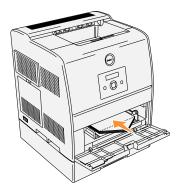
To load envelopes that are under 7.87 inches (220 mm) in width in the multipurpose feeder, insert the envelopes with the flaps open and toward the front of the printer. To load envelopes that are over 7.87 inches (220 mm) in width in the multipurpose feeder, insert the envelopes with the flaps closed and the short-edge of the envelopes facing into the printer. You can load envelopes up to the maximum fill line in the tray at one time.
